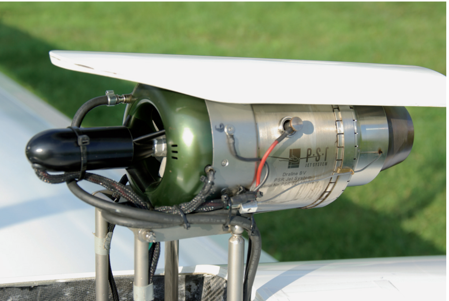
Above: The PSR To1-Turbine supplies 230 N Thrust, the competitors offer up to 400 N
