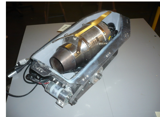
Propulsion system including the withdrawable unit
